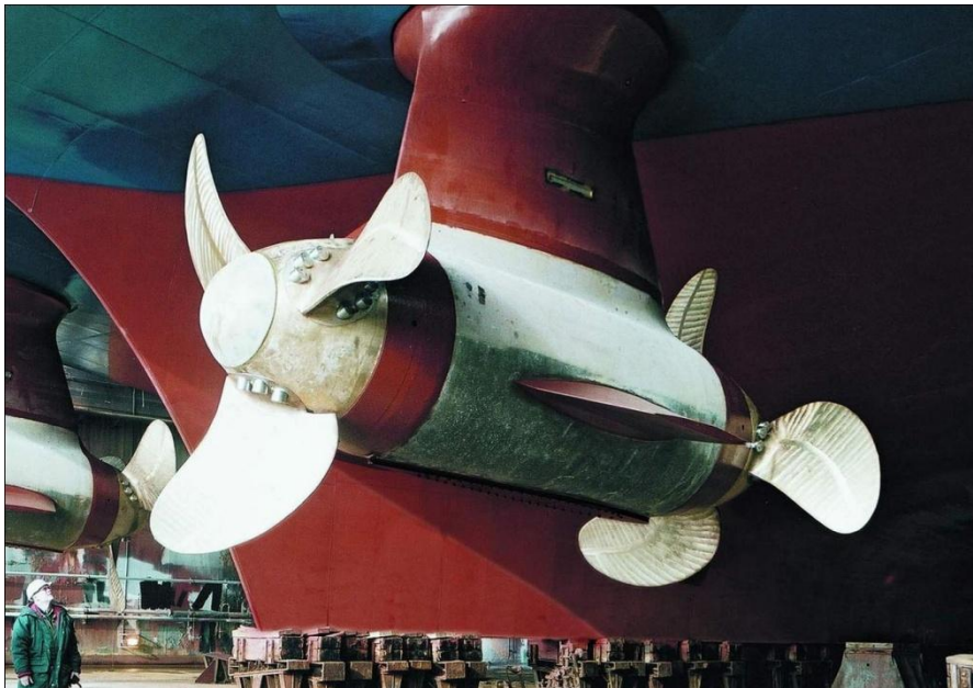
Fig.2. Siemens-Schottel arrangement of pod drive
