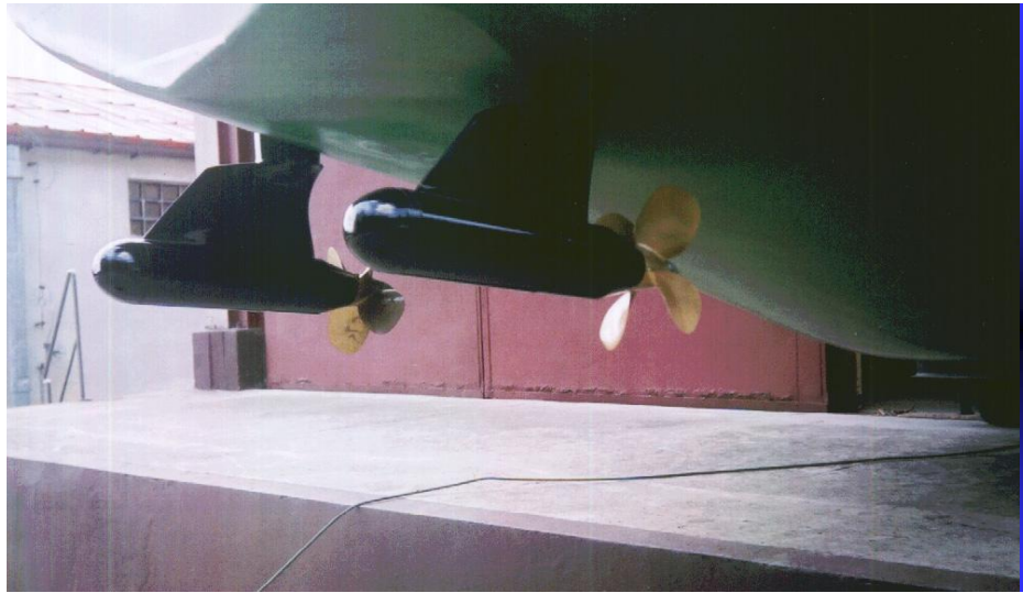
Fig.10. Gas carrier model converted from twin-screw to azipod drive (SRTC)
