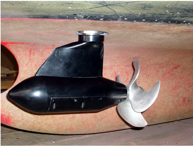
One of the two 21.5 MW pods installed on the Normandie
