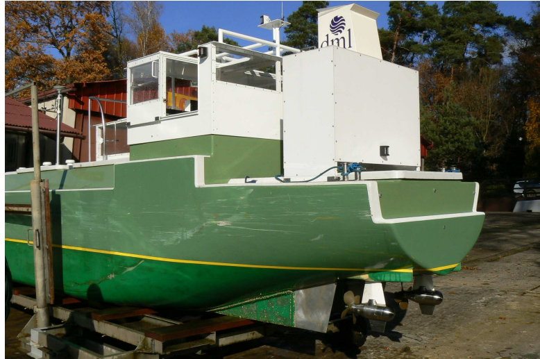
photo no 1: the azipod propulsion installed onboard the training model of a LNG carrier
