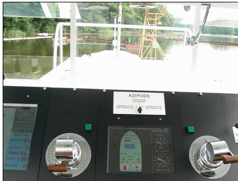
photo no 2: control desk of the pod system of propulsion
