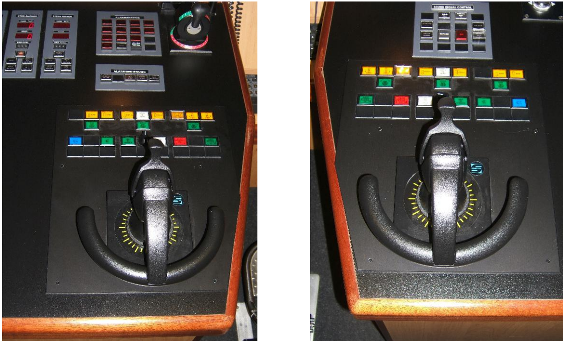
Fig 8 – Final installation of the ACD handles for the Schottel propulsion
