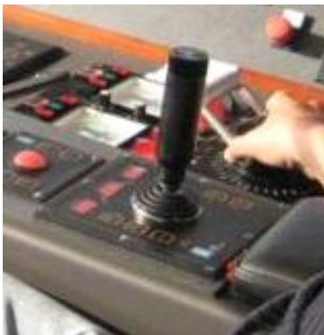
Joystick on the inland vessel “Futura Carrier” 23
