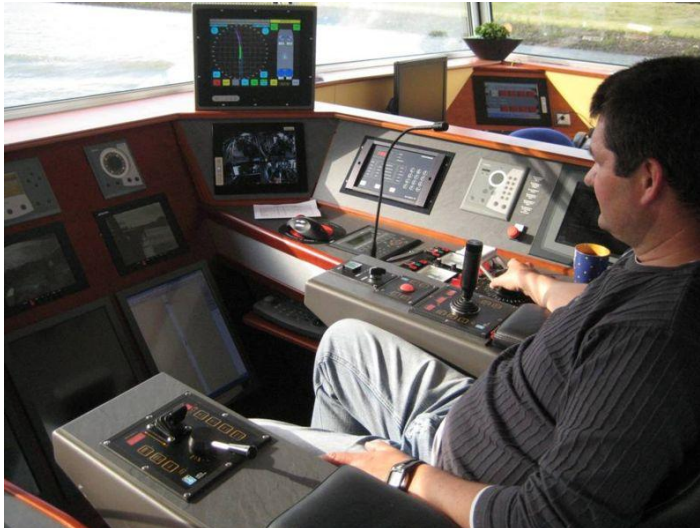
Rudder handle, Joystick and polar handle on the inland vessel "Futura Carrier" 25
