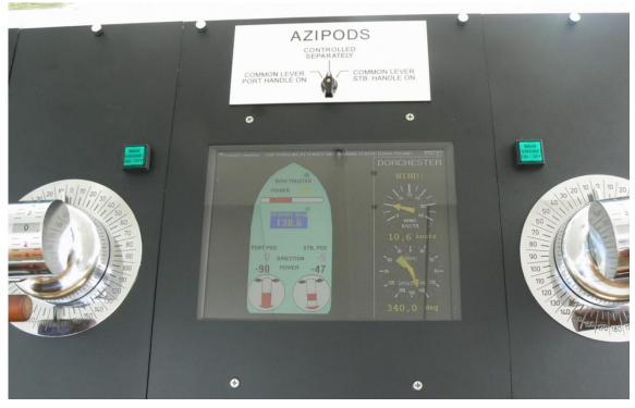
Fig.6. Control desk of the model of gas carrier in SHRTC
