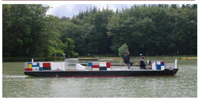
Fig 2. Model of container vessel with azimuting propulsion (Port Revel Shiphandling)
