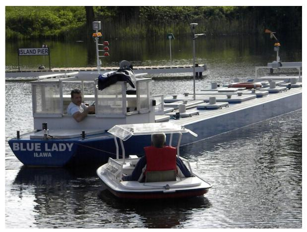
Fig.9. POD driven tug model working with the tanker model at SHRTC
