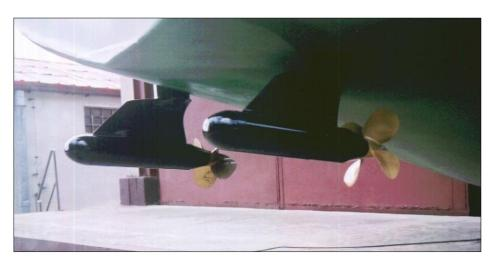
Fig.5 POD propellers in the model of gas carrier in SHRTC
