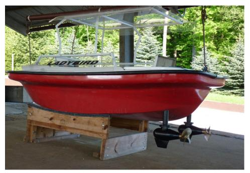
Fig. 7. POD driven tug used in SHRTC
