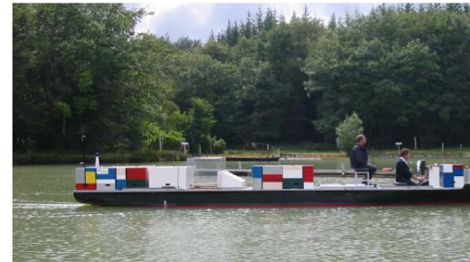
Fig 2. Model of container vessel with azimuthing propulsion (Port Revel Shiphandling)
