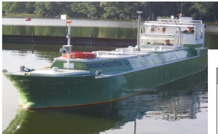
Fig.4. Model of POD driven gas carrier in SHRTC
