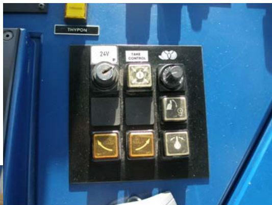
Close up photo of push buttons for taking control from levers to push buttons
